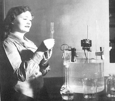
Moira uses an Ostwald Viscometer to determine viscosity
